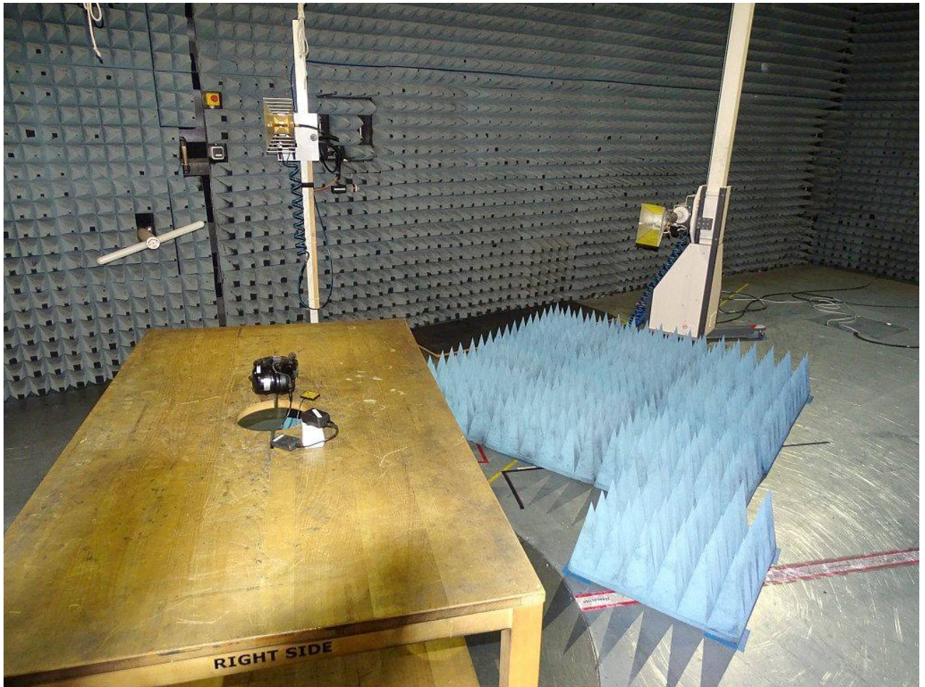
Photo 6: Test setup for radiated measurements above 1 GHz (AC Port (power line), EUT supplied by AC/DC adapter, unintentional radiator §15.109, ANSI C63.4); the test antenna is on the right side mounted at the boresight-mast.
