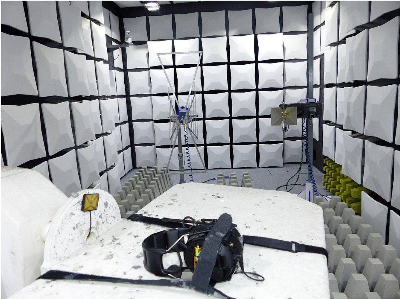
Photo 3: Test setup for radiated measurements (Enclosure, fully-anechoic chamber, 1-25 GHz intentional radiator §15, ANSI C63.10)
