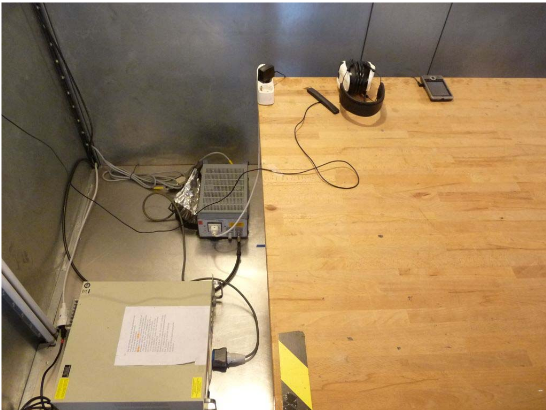
Photo 4: Test setup for conducted measurements (AC Port (power line))
