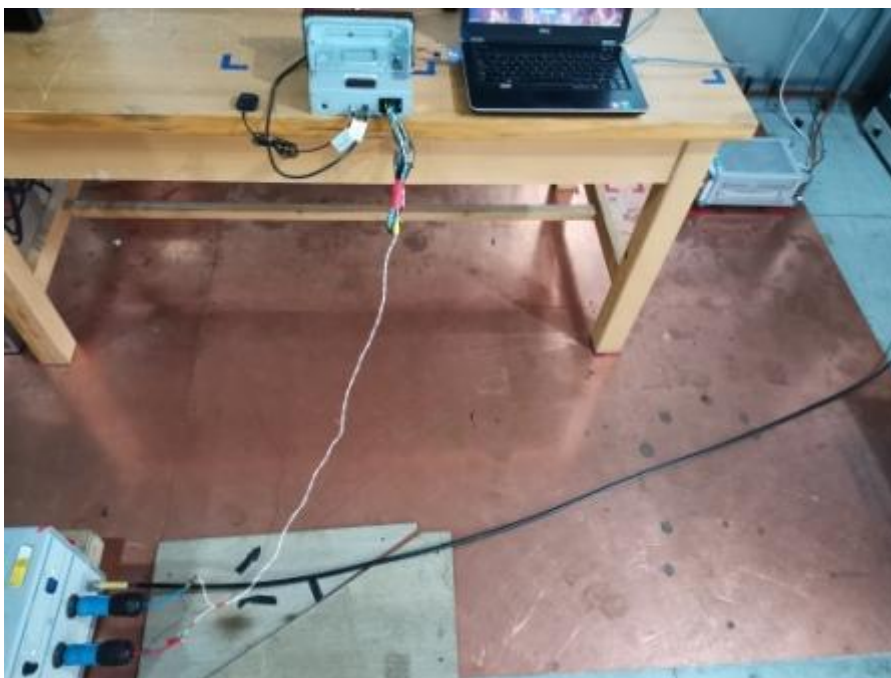
Conducted Emissions Test Setup (with charger)
