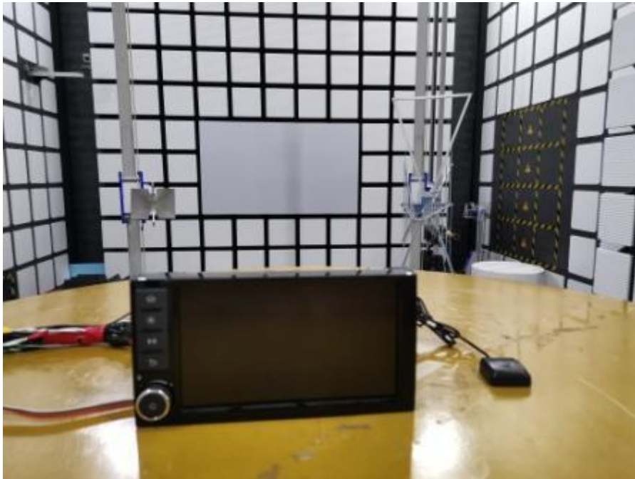
Spurious Radiated Emissions Test setup
