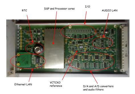
This board can process up to 8 analogical duplex signals ensuring 70 dB of SNR; it can manage 16 logical signals which can be configured both as input and output.
