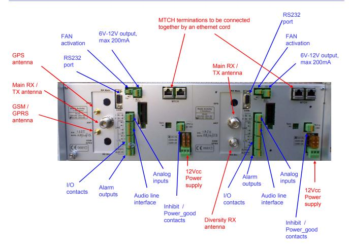
For this example, the following picture shows how two repeaters should be connected to implement a simulcast network with UHF links. Two ethernet patch cord are needed to connect together the MTCH ports and the ethernet ports of the two radios; they are represented in pink color.
