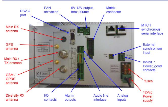
The following connections are available (for each one, a picture of the connector and the related schematic diagram of back plane PCB are shown):
