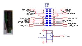
SYNC IN: a MCX coaxial connector for eventual external synchronization input signal. Normally this input is unused, it is needed for special applications which require an external synchronization source (sinusoidal, at 12.8MHz, with level between -10 and 0 dBm).
