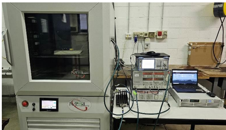
Set-up photo for frequency error tests
