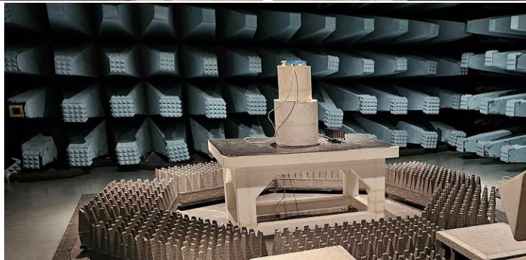
Set-up photo for radiated tests above 1 GHz photo
