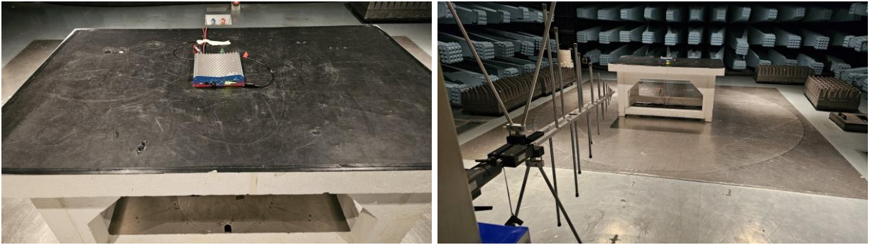
Set-up photo for radiated tests below 1 GHz photo
