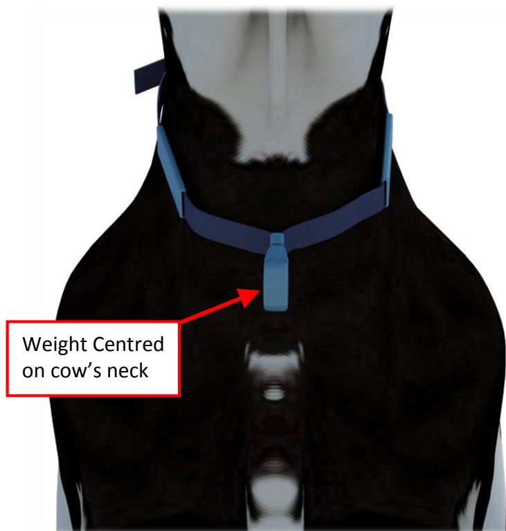
Figure 29 - Typical View of the MooMonitor installed on the cow. (The Weight should be centred on the cow's neck to ensure the MooMonitor stays in position)
