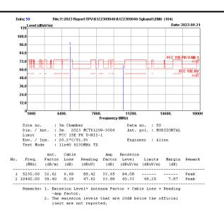
Data: <mark>51</mark> File: F:\2023 Report\TPV\A1Z2309040\A1Z2309040-5gband1.EM6 (104) Date: 2023-09-21 120 Level (dBuV/m) 108.0 96.0 84.0 FCC 15E PK U-NII-72.0 ₽₩₽₽ 101-00 п 60.0 48.0 36.0 24.0 12.0 0 1000 7800. T Frequency (MHz) 11200. 18000 4400. 14600. Site no. : 3m Chamber Dis. / Ant. : 3m 2023 MCTD1209-3006 Limit : FCC 15E PK U-NII-1 Env. / Ins. : 20.2\*\*(51.5% Test Mode : 11n40 5230MHz TX Data no. : 51 Ant. pol. : VERTICAL Engineer : Allen
