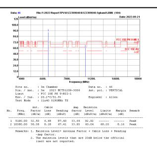
Data: 47 File: F:\2023 Report\TPV\A1Z2309040\A1Z2309040-5gband1.EM6 (104) Date: 2023-09-21 120 Level (dBuV/m) 108.0 96.0 84.0 FCC 15E PK U-NII-72.0 ┱╓┢╻ in n п 60.0 48.0 36.0 24.0 12.0 0 1000 7800. 1 Frequency (MHz) 11200. 18000 4400. 14600. Site no. : 3m Chamber Dis. / Ant. : 3m 2023 MCTD1209-3006 Limit : FCC 15E PK U-NII-1 Env. / Ins. : 20.2\*\*(51.5% Test Mode : 11n40 5190MHz TX Data no. : 47 Ant. pol. : HORIZONTAL Engineer : Allen
