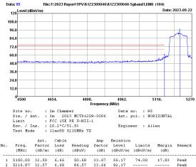
50.68 33.67 56.17 86.57 33.66 92.17 5150.00 32.50 6.66 5216.87 32.57 6.69 1 2 Peak Peak Remarks: 1. Emission Level= Antenna Factor + Cable Loss + Reading -Amp factor.
