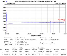
76.08 33.68 33.54 83.07 33.88 43.97 5823.40 33.60 7250.00 36.70 6.93 7.47 1 Average Average 54.00 10.03 Remarks: 1. Emission Level= Antenna Factor + Cable Loss + Reading -Amp factor.
