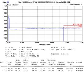
54.00 Remarks: 1. Emission Level= Antenna Factor + Cable Loss + Reading -Amp factor.
