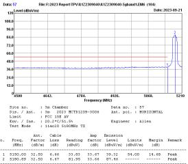
Remarks: 1. Emission Level- Antenna Factor + Cable Loss + Reading -Amp factor. 2. The emission levels that are 20dB below the official limit are not reported.
