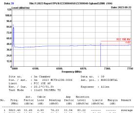
76.23 33.81 5823.40 33.60 7250.00 36.70 83.22 44.10 6.93 7.47 33.54 33.88 1 Average Average 54.00 9.90 Remarks: 1. Emission Level= Antenna Factor + Cable Loss + Reading -Amp factor.
