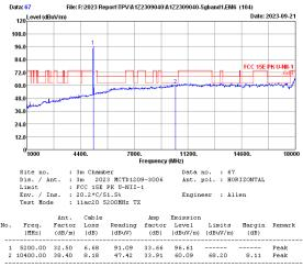
Remarks: 1. Emission Level = Antenna Factor + Cable Loss + Reading -Amp factor.
