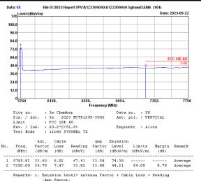
Remarks: 1. Emission Level- Antenna Factor + Cable Loss + Reading -Amp factor. 2. The emission levels that are 20dB below the official limit are not reported.
