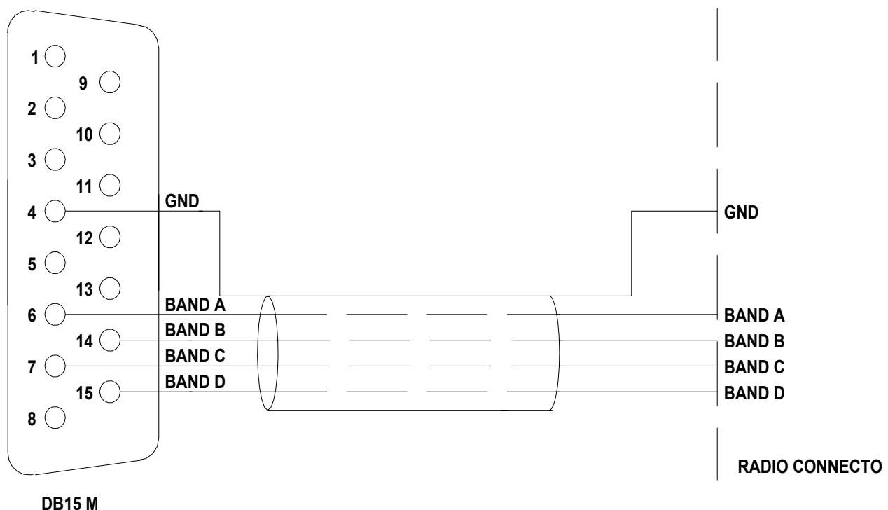
Without the CAT, the band is commanded by four digital signals (Band A, Band B, Band C, Band D). Refer to the specific manual.
