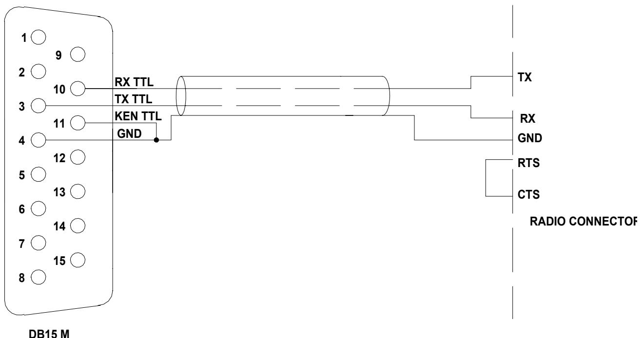
The connector is described in the specific manual. Verify if the RTS–CTS link is necessary.
