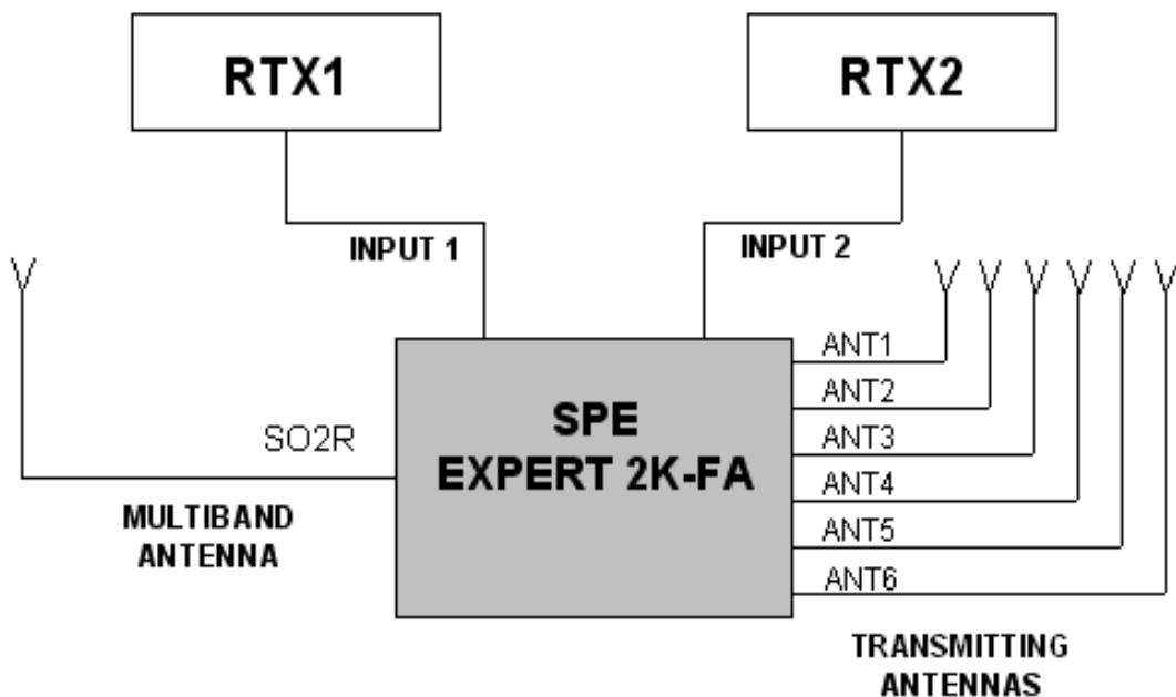
This kind of operation is used during a contest in order to acquire, as quickly as possible, a new multiplier.
