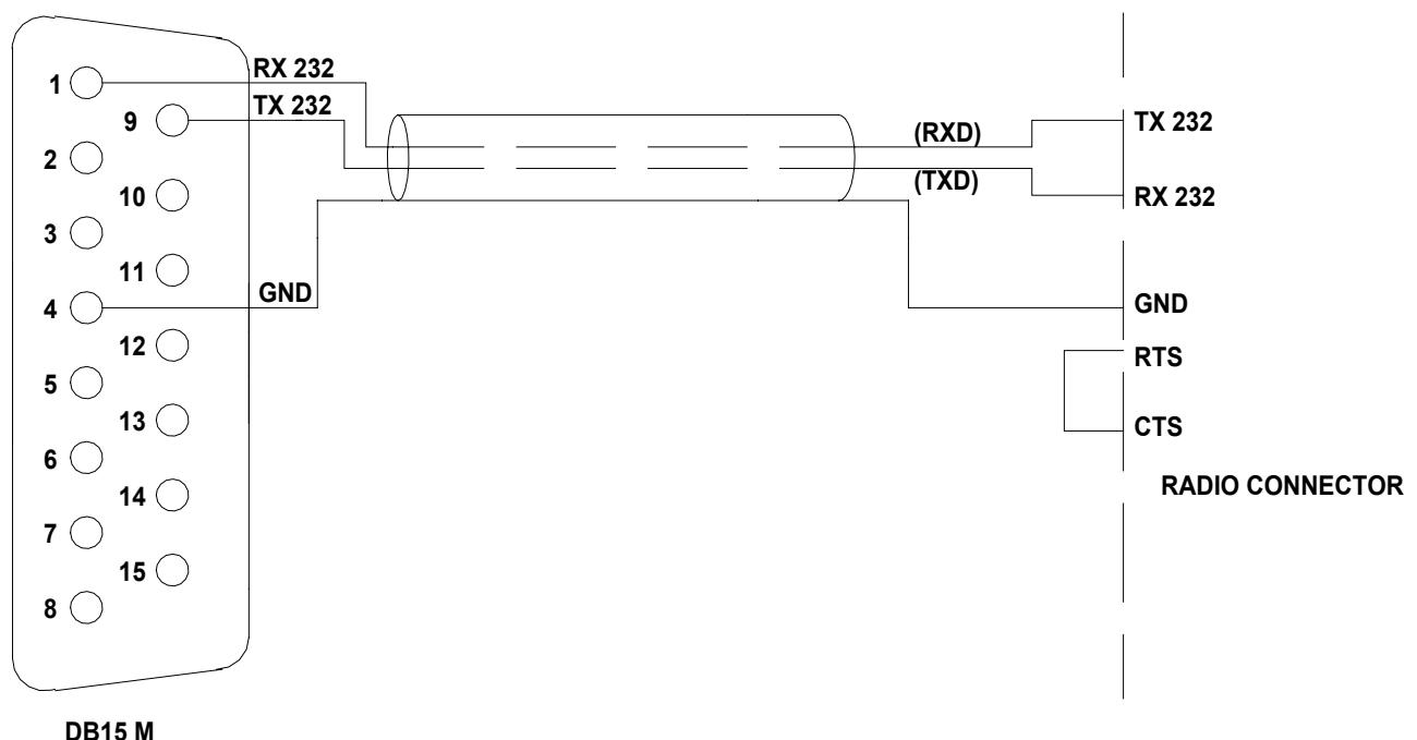
The radio connector may be a DB-9 or DB-25 male connector or female connector (read specific manual). Verify from the manual if the RTS-CTS link is necessary.
