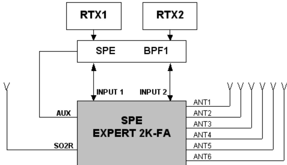
These features can be possible also with the simultaneous use of the unit "SPE SO2R1, (use the **AUX** port with a Y cable).
