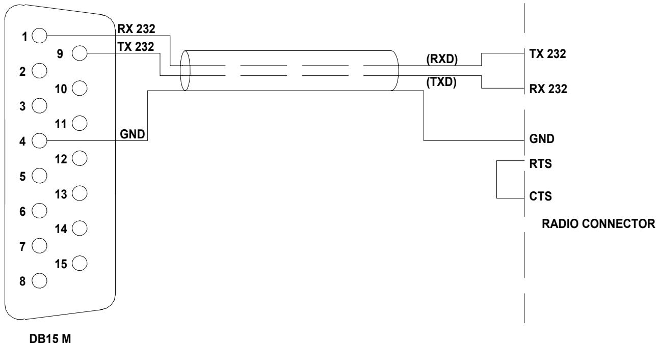
The radio connector may be a DB-9 or DB-25 male connector or female connector (read the specific manual). Verify from the manual if the RTS–CTS link is necessary.
