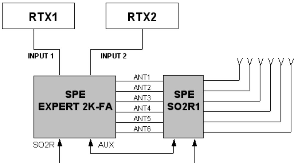
The unit is controlled and powered from the AUX port.
