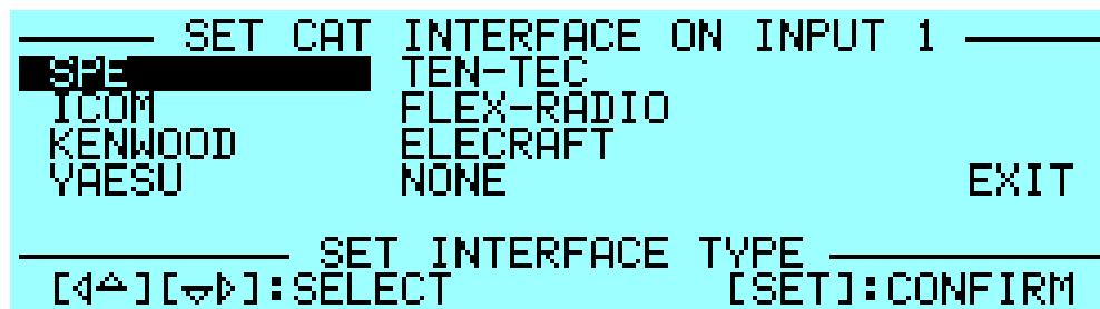
Select the brand or function, for the proper link see "CAT CONNECTIONS" on this manual.
