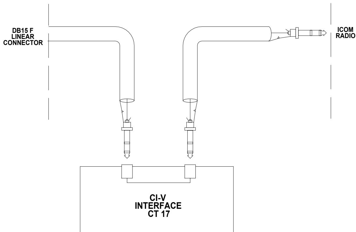
The plug from the amplifier has to be connected to a CI-V port of the CT17 or similar device. The transceiver has to be connected to another CI-V port.
