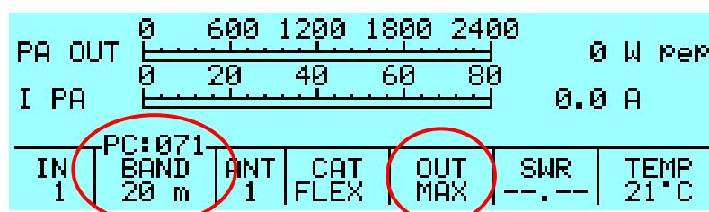
Pressing the arrow keys ([◀▲] [▼▶]) this value can be decremented/incremented until it reaches the requested value; at the operation completion a time-out period (about 3 seconds) must be awaited for the “[PC=xxx]” indication to expire to permit another adjustment to be made.
