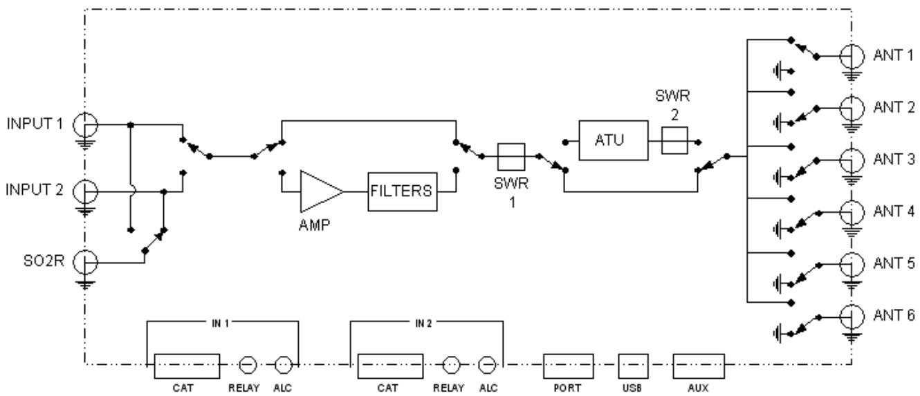
The position of the contacts, as shown in the diagram, is the situation of the linear amplifier in OFF state.
