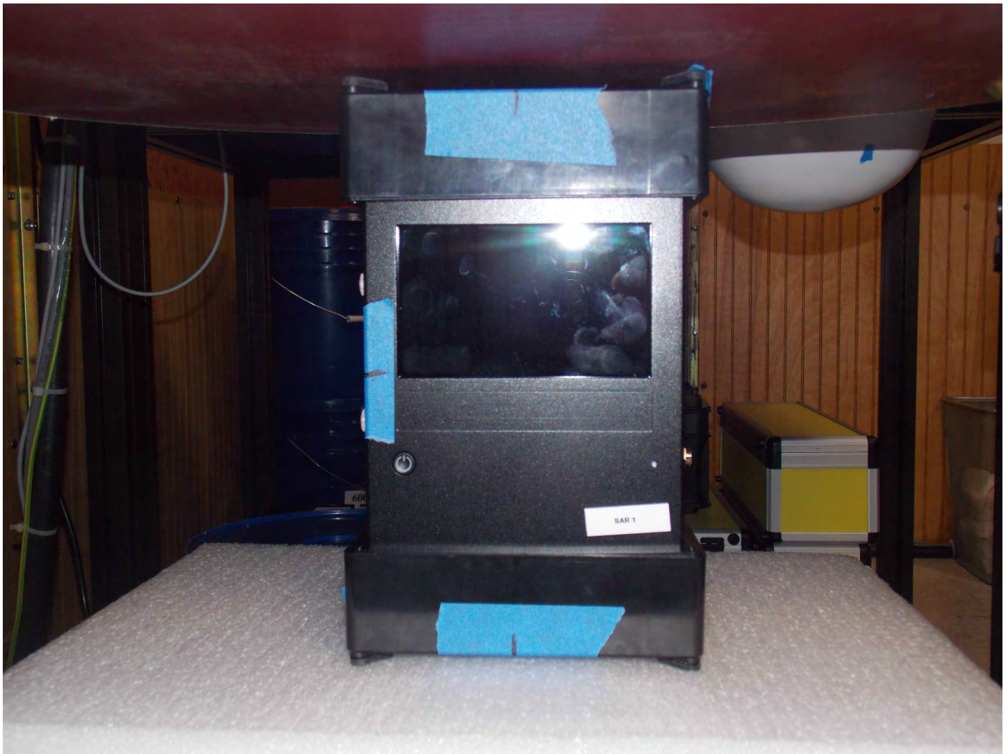
Test Position Top 10 mm Gap
