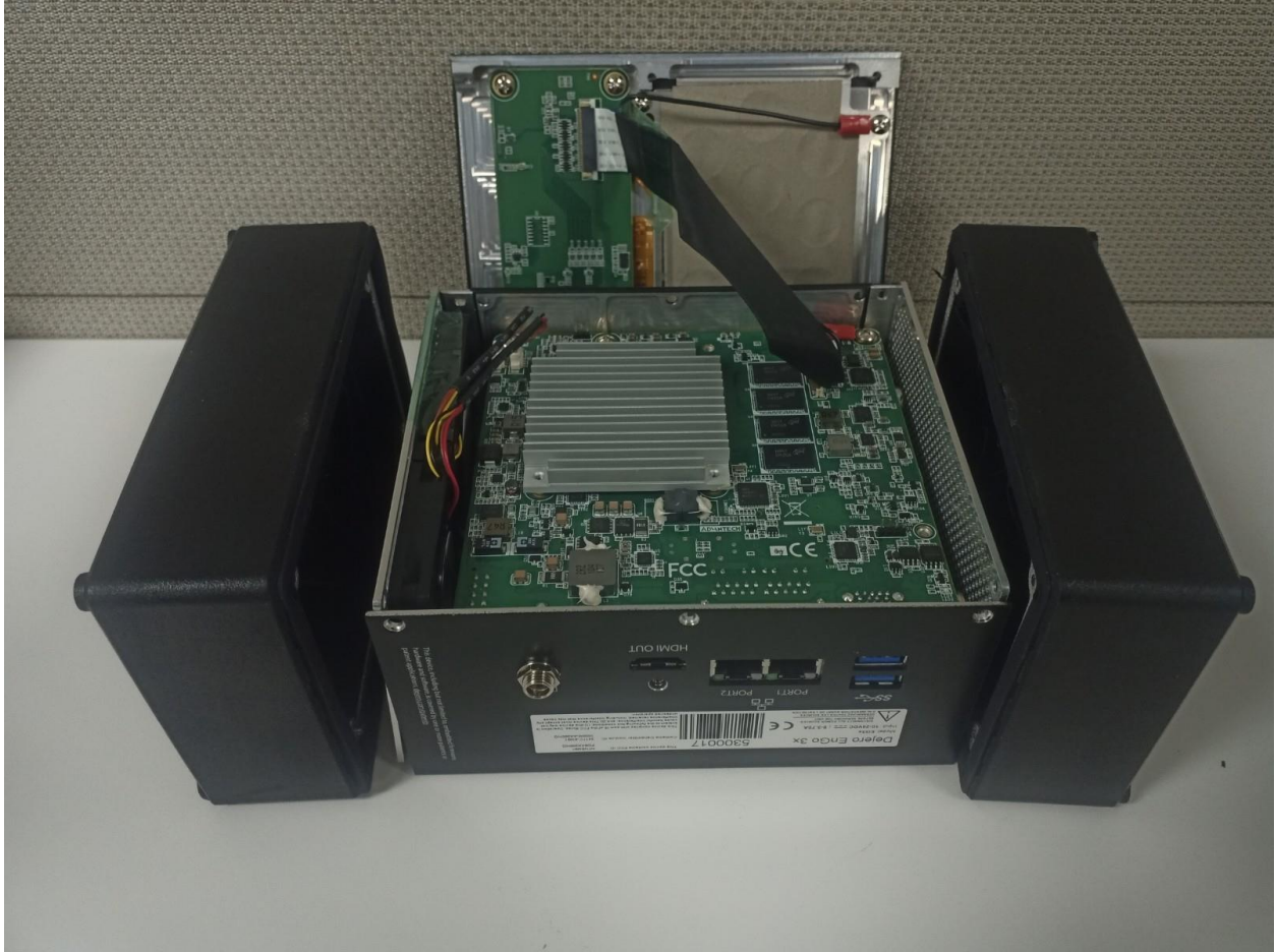
Front cover/screen removed with device facing up. Endcaps detached.
