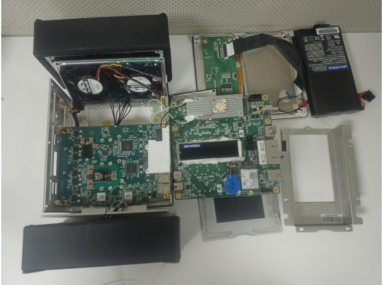
Device facing down, battery removed, screen removed, battery tray removed, endcaps detached, SBC disconnected from RF board.
