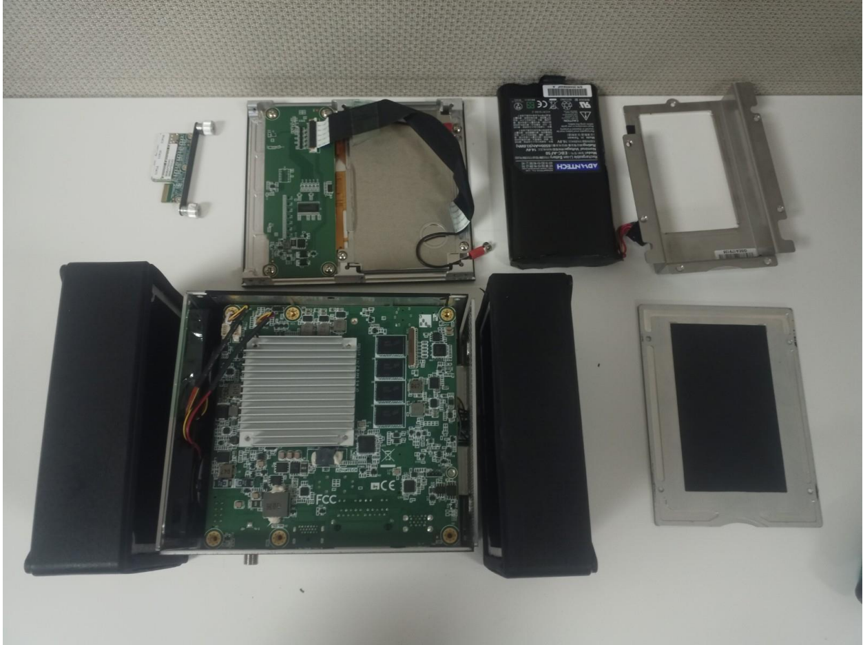
Device facing up, battery removed, screen removed, battery tray removed, endcaps detached, SBC (Single Board computer) showing.
