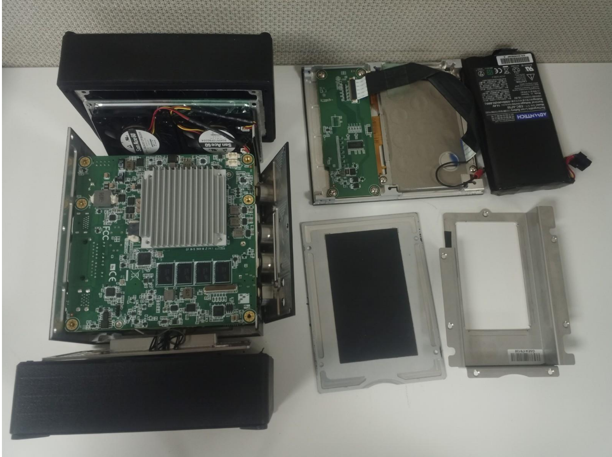
Device facing down, battery removed, screen removed, battery tray removed, endcaps detached, I/O plate loosened.
