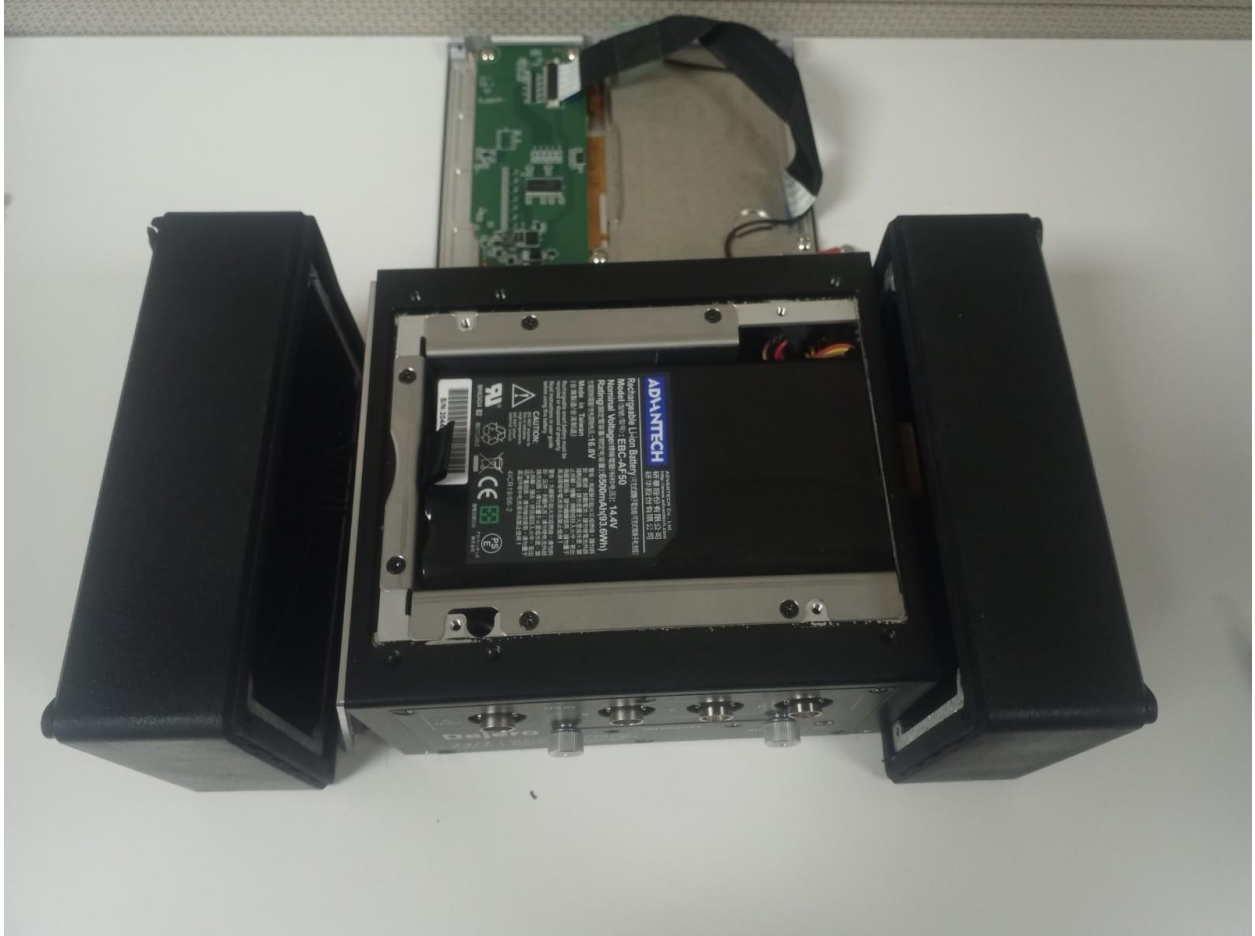
Device facing down, endcaps detached, back cover removed and screen removed.
