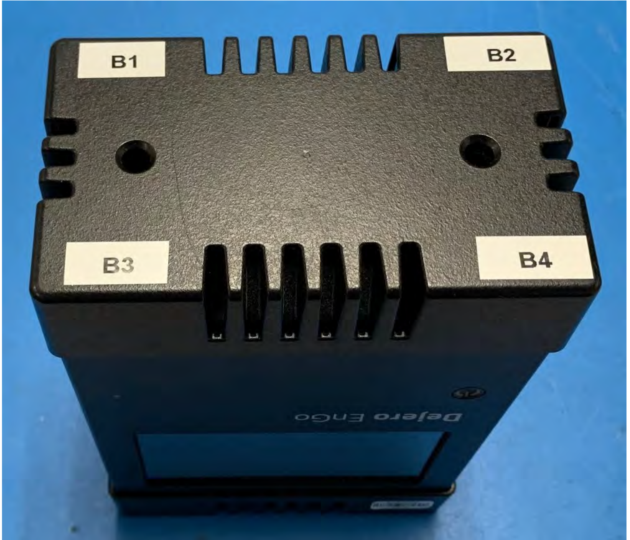
Antennas Located at the Bottom of the Unit
