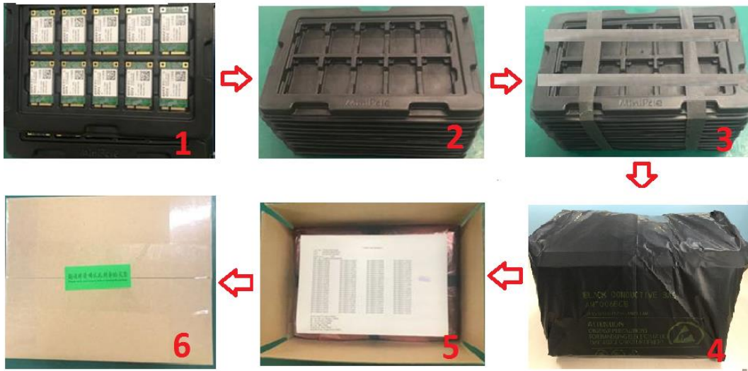
Figure 34: Tray Packaging Procedure
