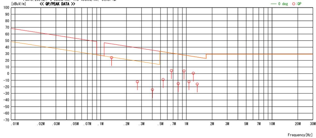
CHART: WITH FACTOR, ANT TYPE: LOOP, Except for the data below: adequate margin data below the limits.
