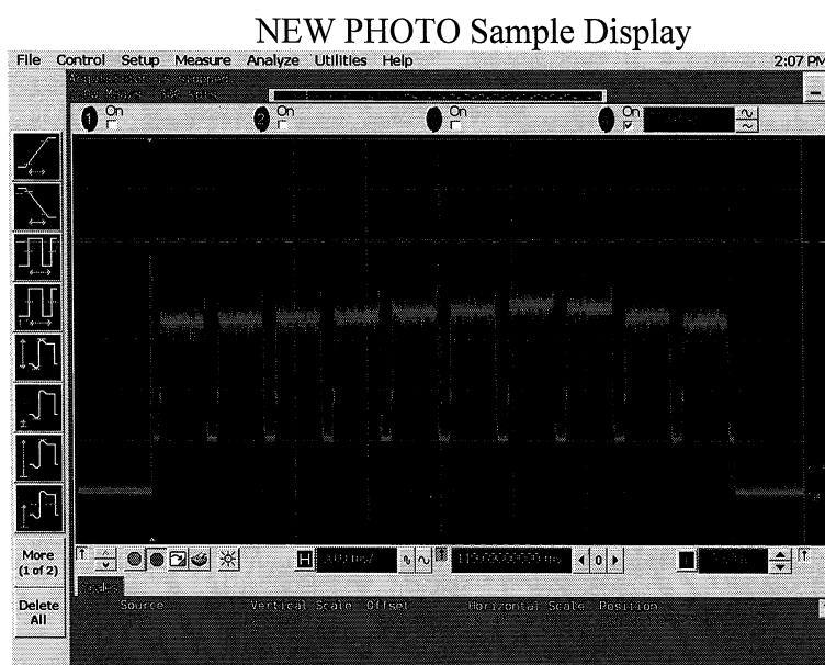
Figure 1. J6 Pin 12 RSSI. 30 msec/div. 200 mV/div AD8310 Output to MCU ADC. No RF Input.
