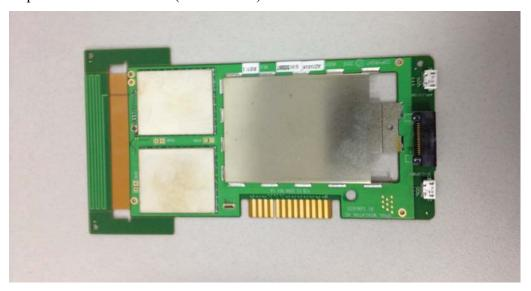
Bottom of Basestation board (with battery):
