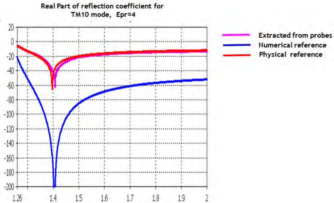
Figure 3-3: Comparison of simulated, physical and numerical references for reflection coefficient of TM mode
