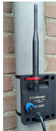
Example of using cable ties to mount the WIB2000 on a pole.
