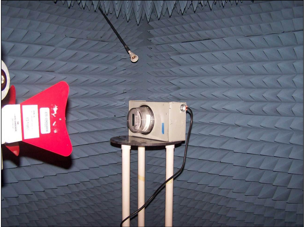
Photograph 2. Radiated Spurious Emissions Test Setup
