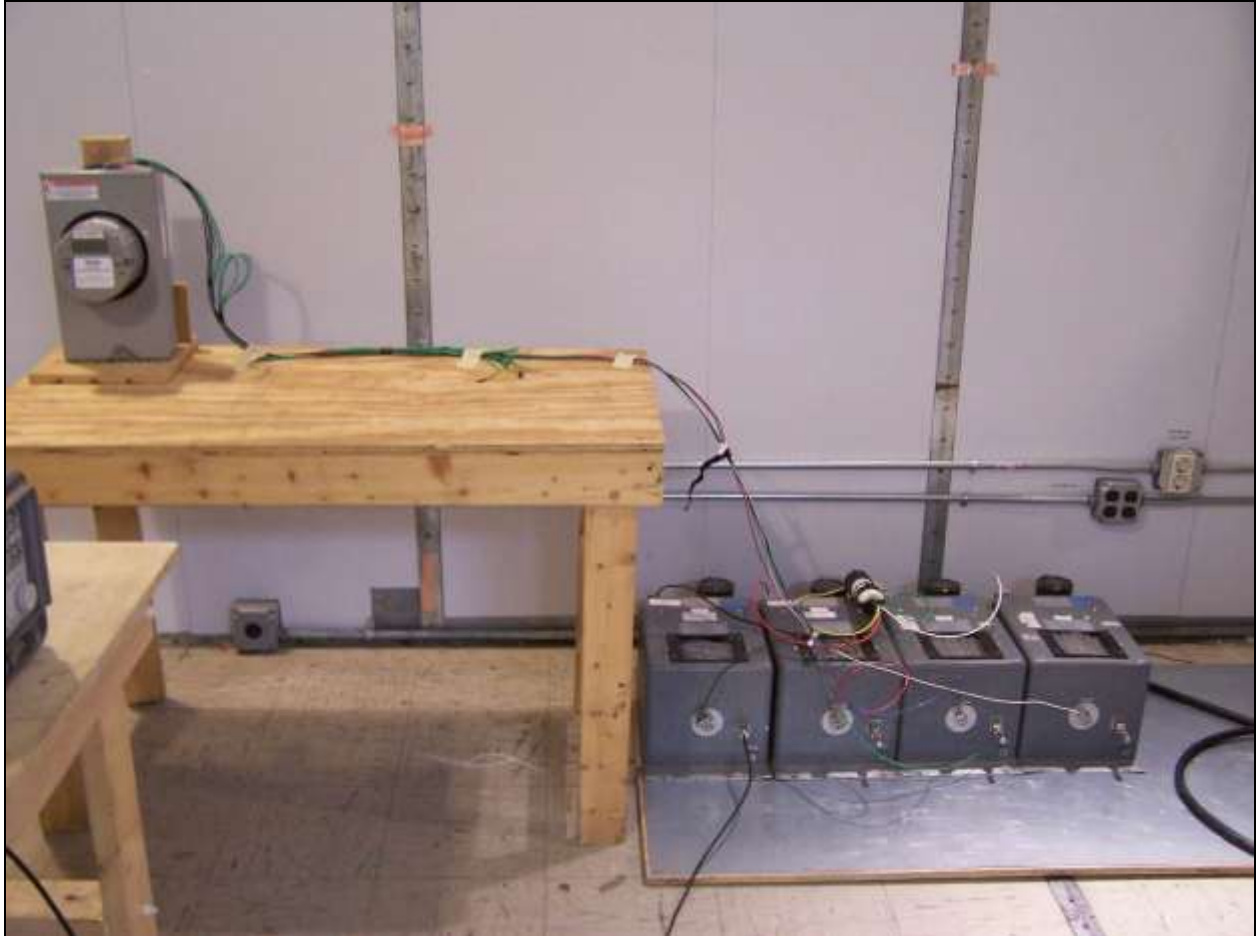
Photograph 2. Conducted Emissions, 15.207(a), Test Setup
