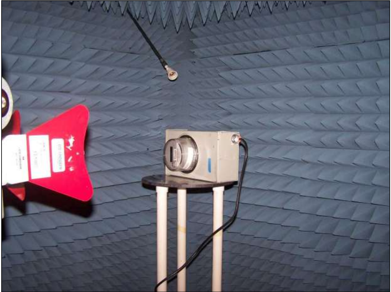
Photograph 3. Radiated Spurious Emissions Test Setup
