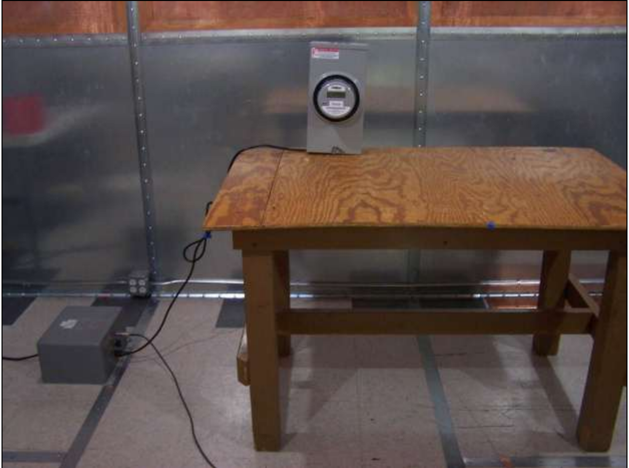
Photograph 2. Conducted Emissions, 15.207(a), Test Setup
