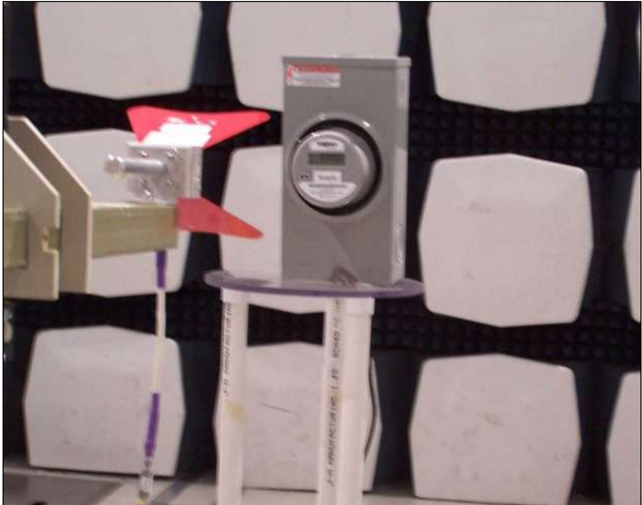
Photograph 3. Radiated Spurious Emissions Test Setup
