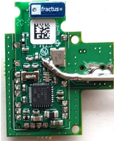
Figure 3 BLE module and interface board 3080043.027 v0.3
