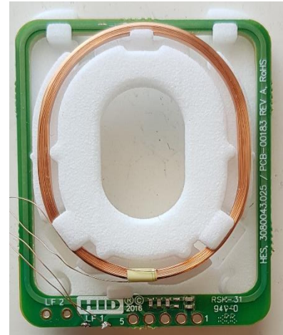
Figure 4 RFID coils assembly (13,56MHz 3080043.025/PCB 00183 v.A)
