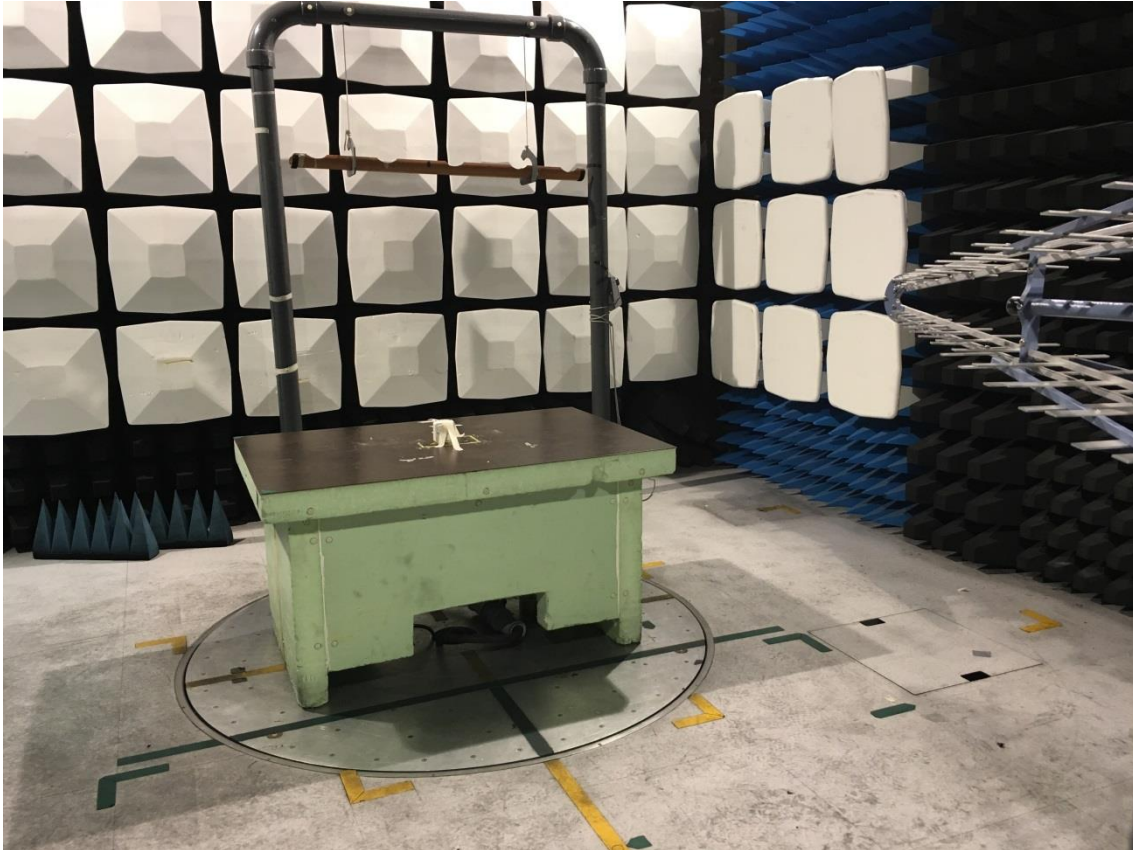
Test set up radiated emission 30 MHz – 1GHz
