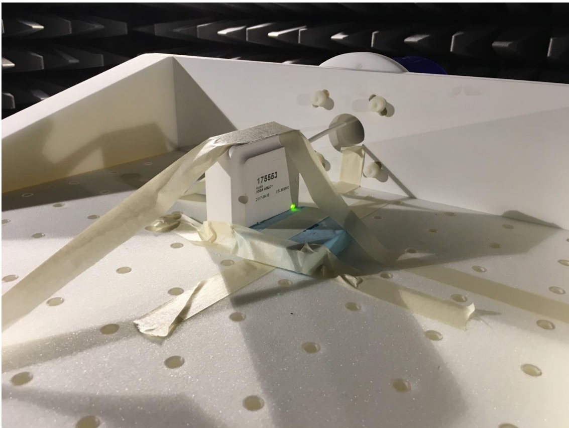
EUT set up radiated emission above 1GHz
