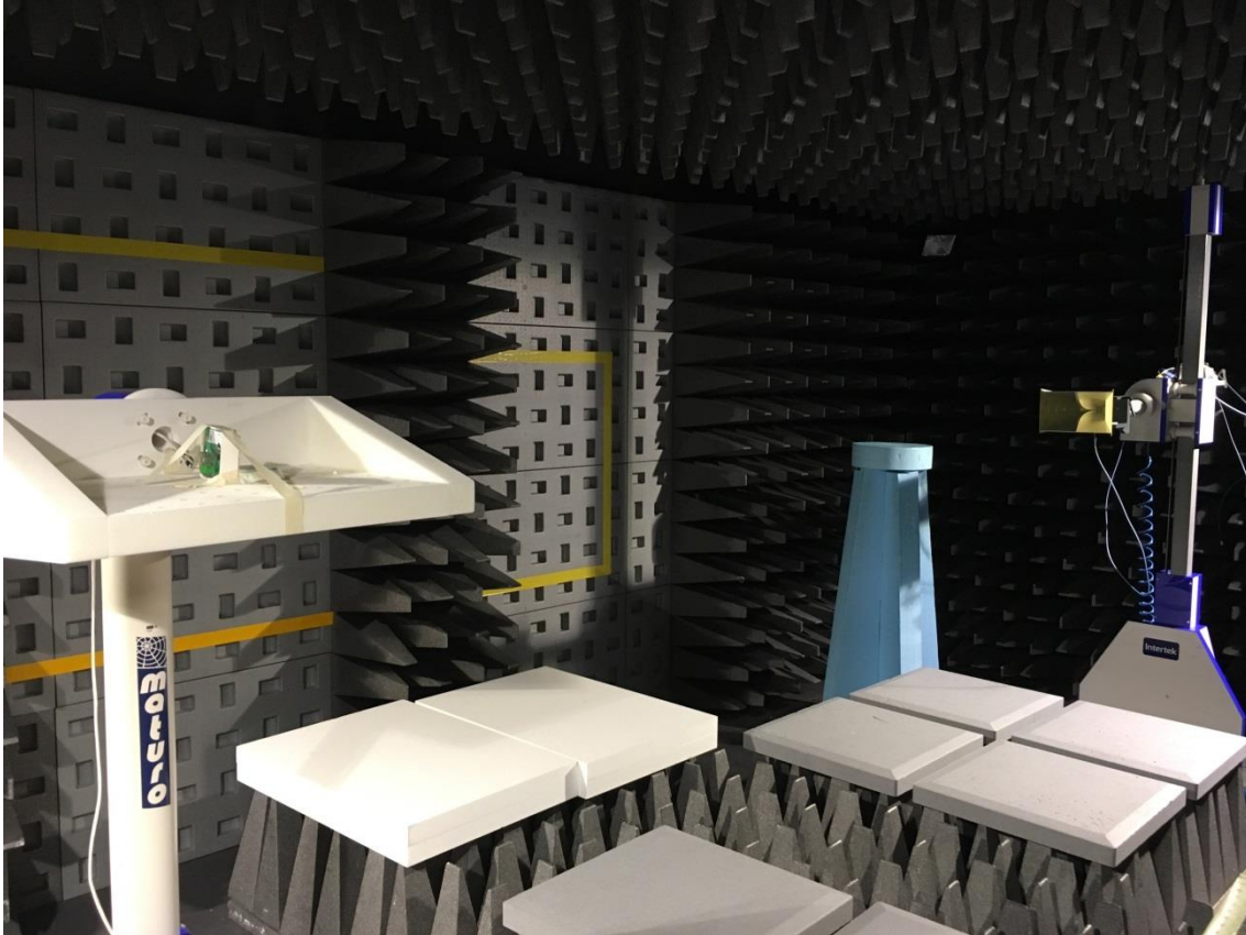
Test set up radiated emission above 1GHz
