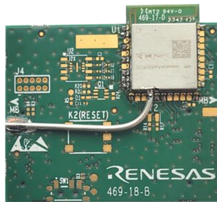
VSWR Renesas DA14592MOD module mounted on reference board.
