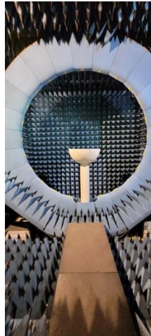
Figure 5-6 Satimo SG-23 6 GHz Stargate Antenna Test Chamber.
