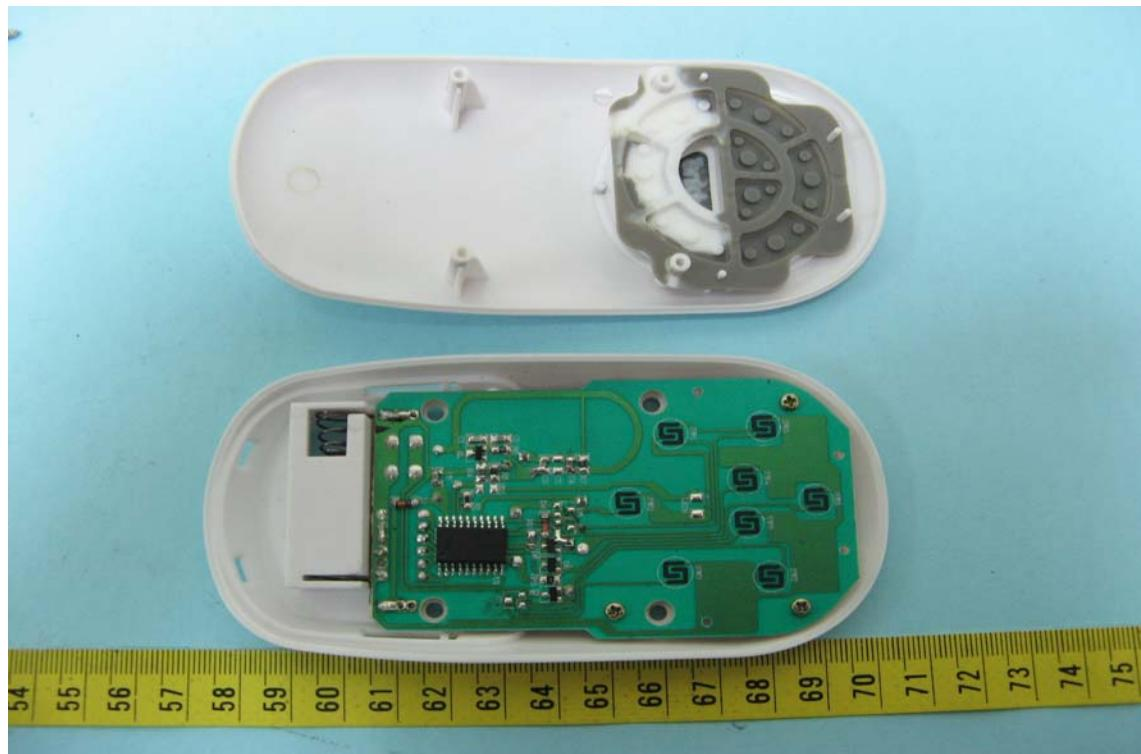
**CONSTRUCTED PHOTOS of EUT****8. Component View of Main PCB**
