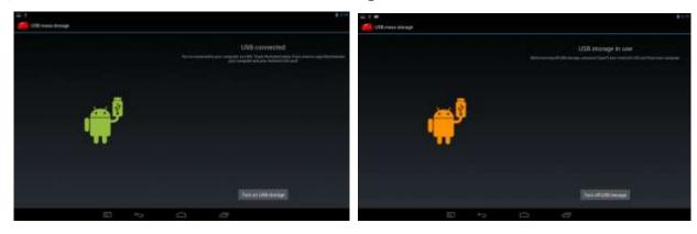
The left picture shows that the device storage content can be viewed and modified from the computer. The right picture means that device storage content can NOT be viewed or modified from the computer.
