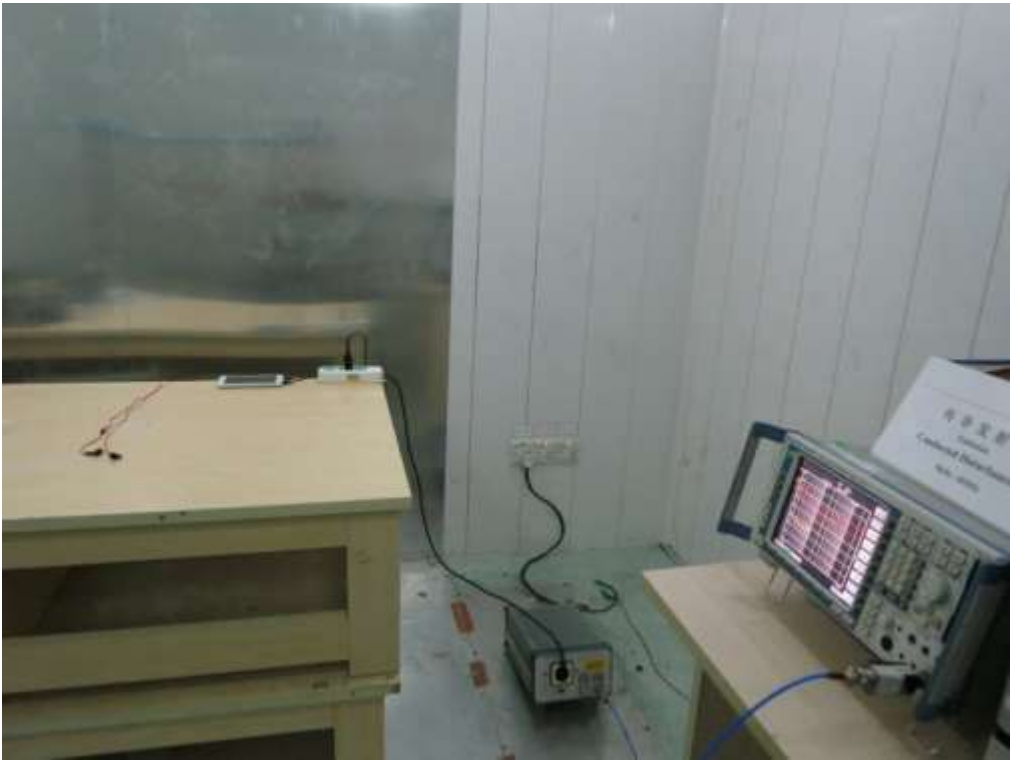
FCC RADIATED EMISSION TEST SETUP
