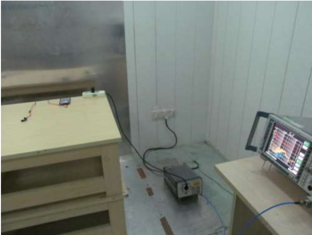
FCC RADIATED EMISSION TEST SETUP
