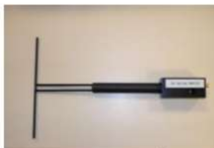
Figure 1 – Satimo COMOSAR Validation Dipole
