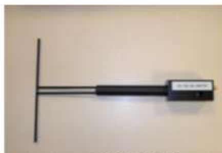
Figure 1 – Satimo COMOSAR Validation Dipole
