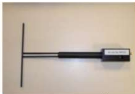
Figure 1 – Satimo COMOSAR Validation Dipole
