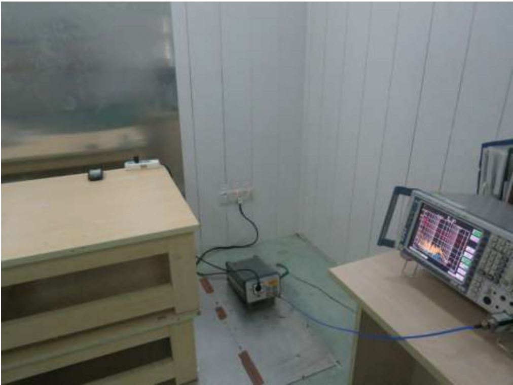
FCC RADIATED EMISSION TEST SETUP
