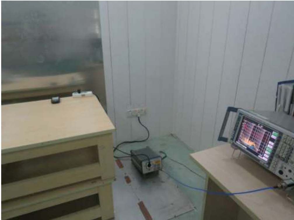
FCC RADIATED EMISSION TEST SETUP
