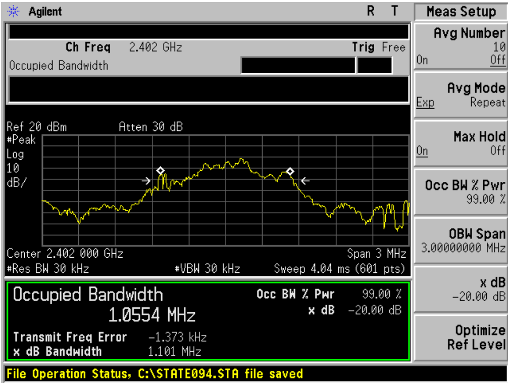
TEST PLOT OF BANDWIDTH FOR LOW CHANNEL
