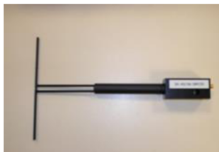
Figure 1 – Satimo COMOSAR Validation Dipole
