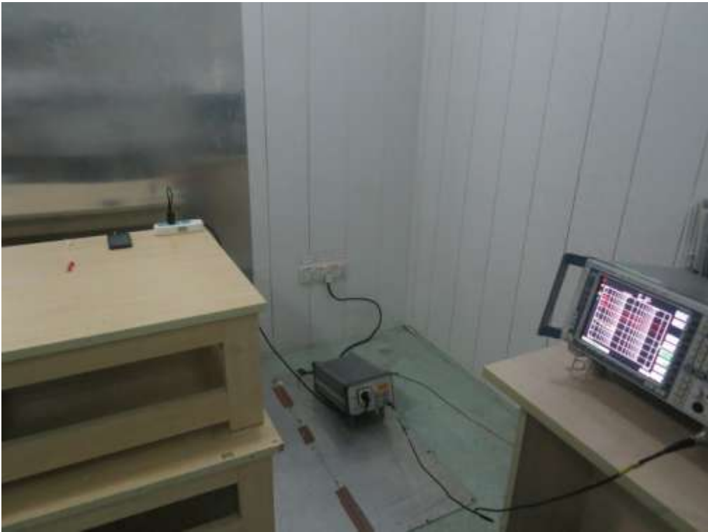
FCC RADIATED EMISSION TEST SETUP
