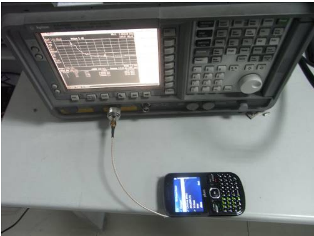
CONDUCTED SPURIOUS EMISSION TEST SETUP
