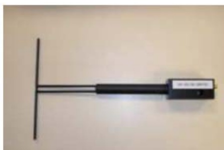
Figure 1 – Satimo COMOSAR Validation Dipole
