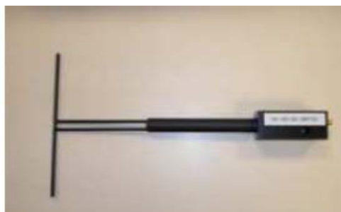
Figure 1 – Satimo COMOSAR Validation Dipole
