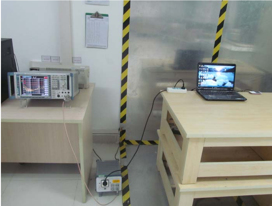
FCC RADIATED EMISSION TEST SETUP
