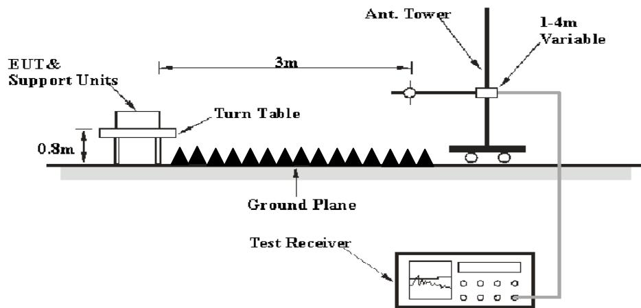
The radiated emission tests were performed in the 3 meters test site, using the setup accordance with the ANSI C63.4-2009. The specification used was the FCC 15.209, and FCC 15.247 limits.
