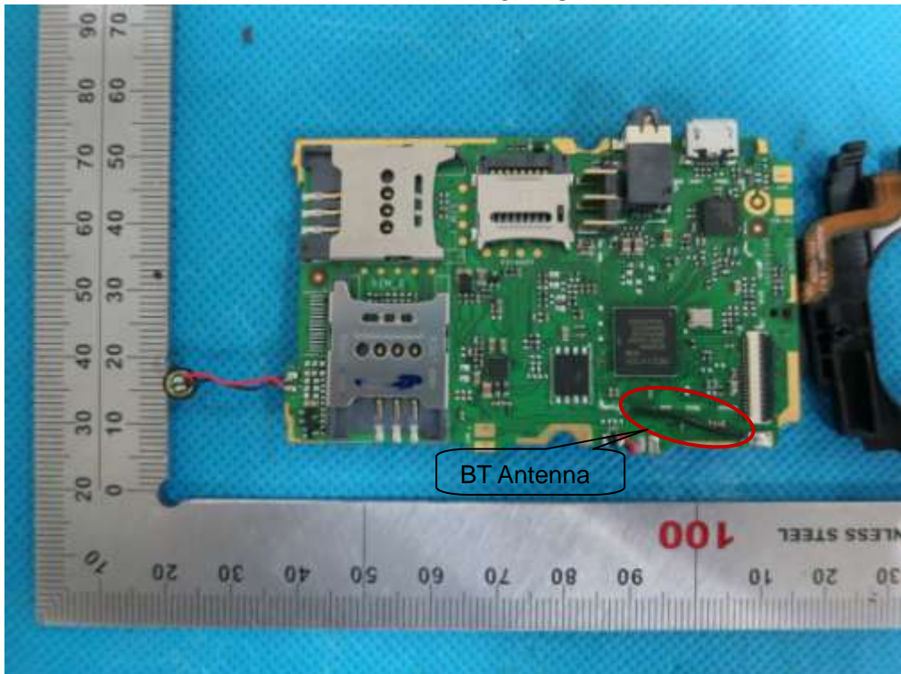
INTERNAL VIEW OF EUT-2
