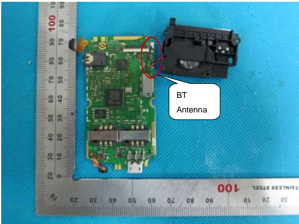
INTERNAL VIEW OF EUT-2
