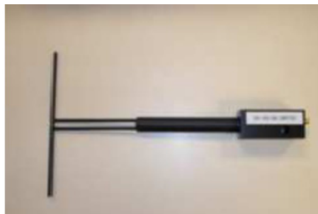
Figure 1 – Satimo COMOSAR Validation Dipole
