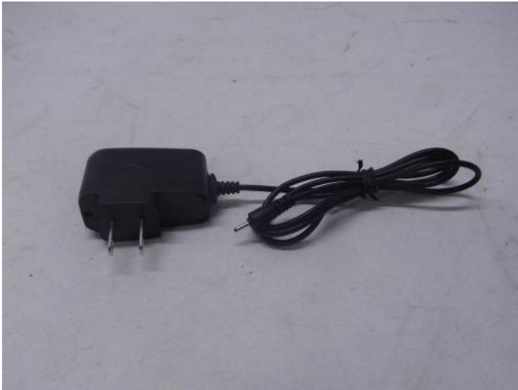
PHOTO OF POWER SUPPLY
