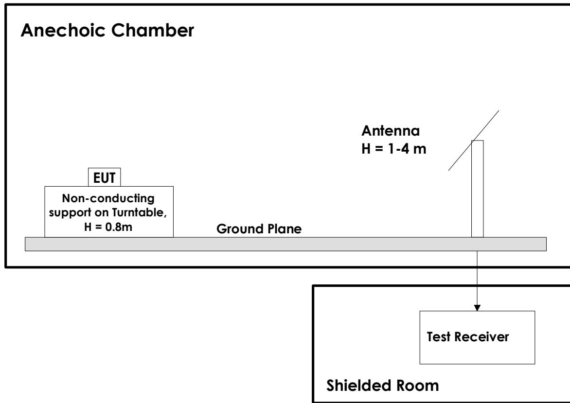
Measurements at 1GHz and above were performed with turntable height 1.5m and with the ground plane covered by absorbers.
