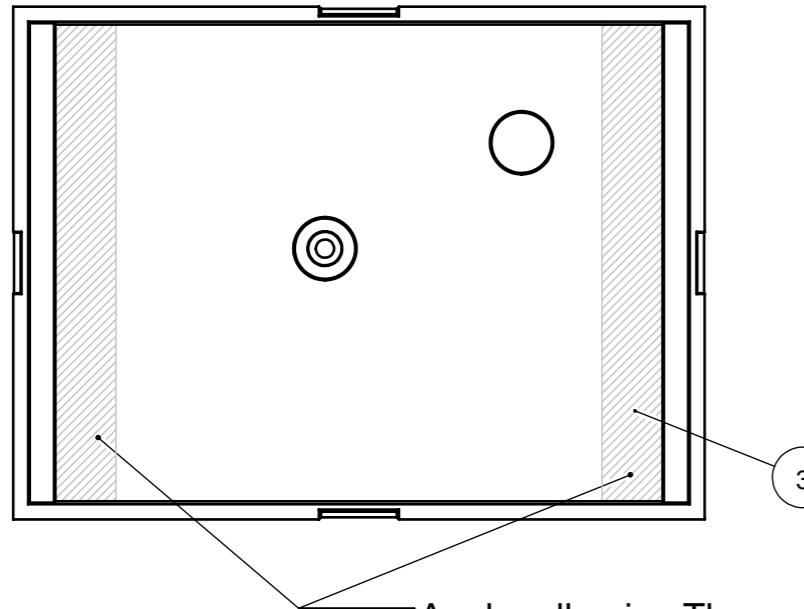
Apply adhesive Theroson MS 939 FR, 4827865, in this area when mounting the PCBA.
