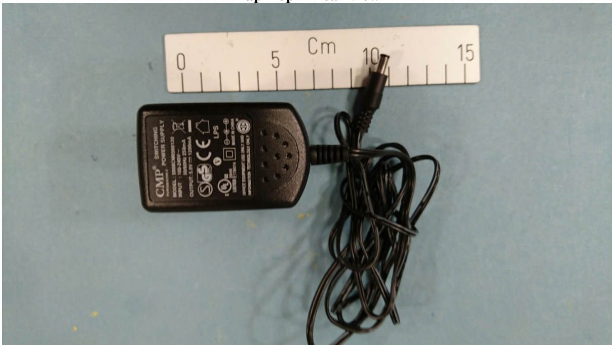
AC/DC adapter for conducted power line measurements.( CMP:S008CM0500120)
