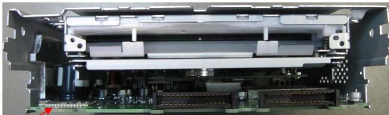
Figure2: MIB Entry Radio without front unit
