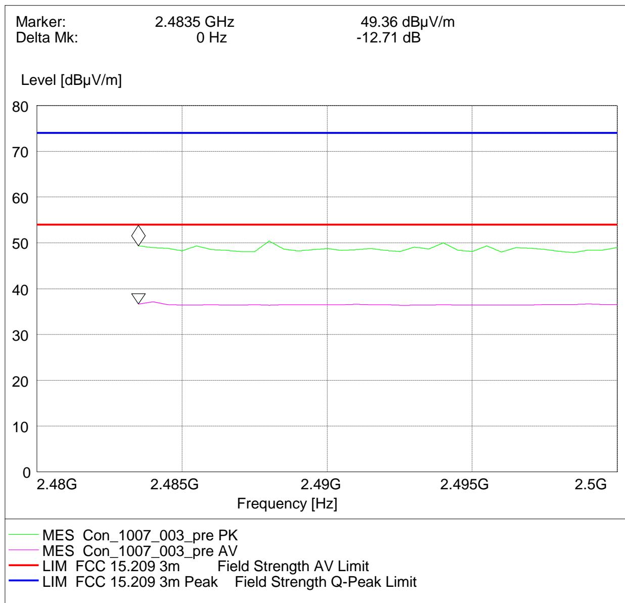
Radiated measurement (higher band edge)
