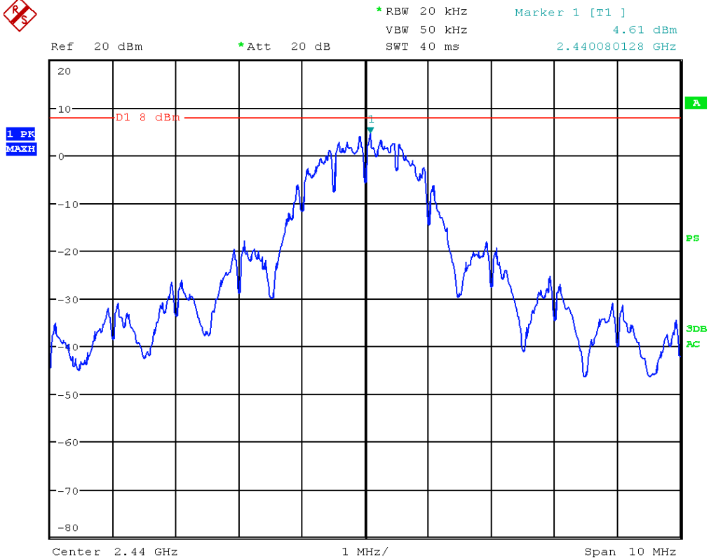
Picture 69: Power spectral density ant01, channel 18 - complete carrier
