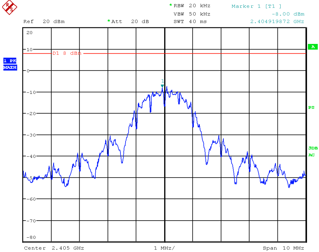
Picture 48: Power spectral density ant00, channel 11 - complete carrier
