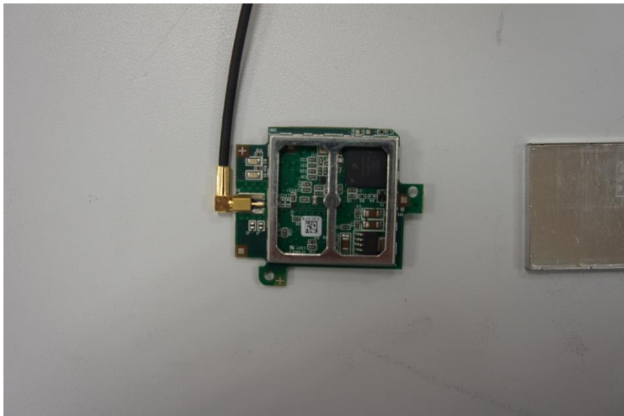
Picture 2: EUT top side without cover
